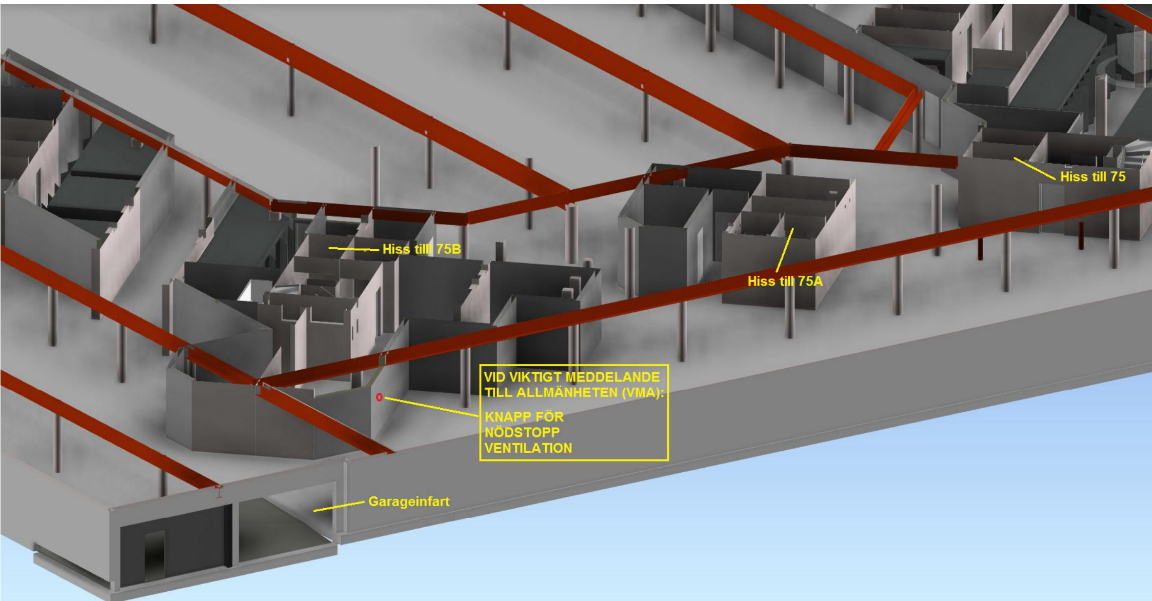
**If emergency stop of ventilation is prohibited (in case of toxic smoke pollution due to nearby fire) a stop-button for the entire ventilation system is located in the garage in the basement, near the entrance. By pushing the button the entire ventilation system for the house stops.**
